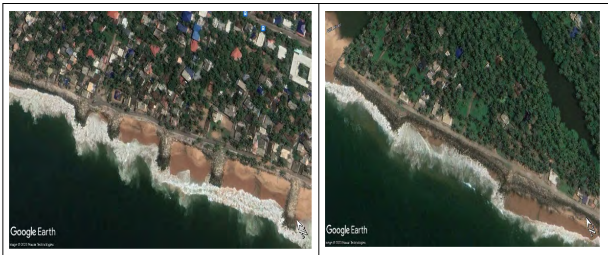
Figure 4-3 Groyne fields north of the port
