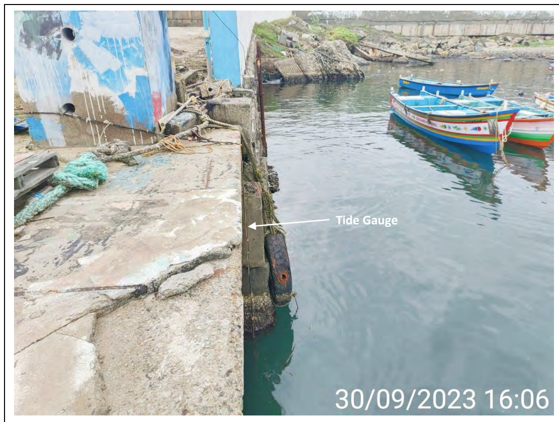
Figure 5-1: Automatic Tide Gauge
