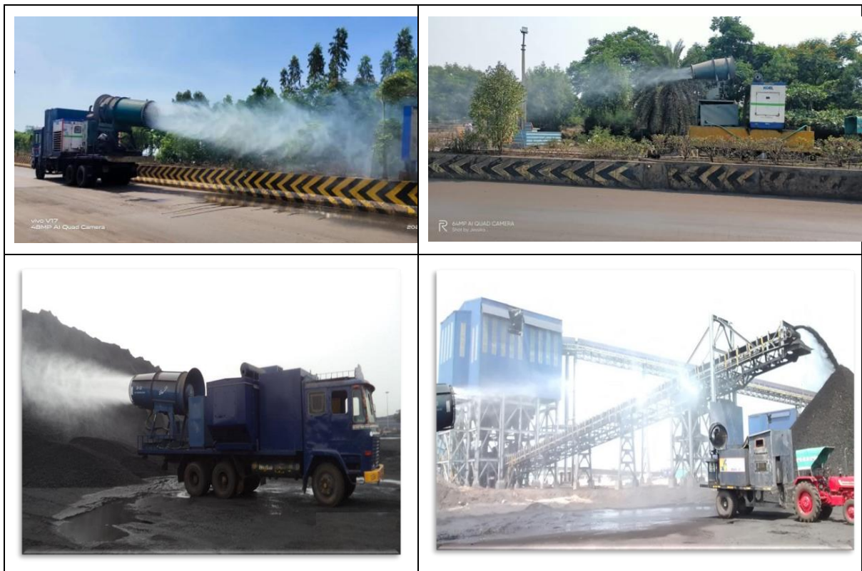
Figure 2:7 Atomizers in dust suppression system
