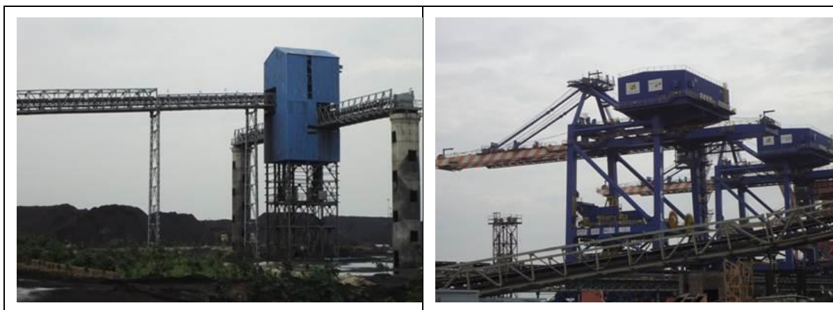
Figure 2:2 Conveyor streams and Grab ship unloaders
