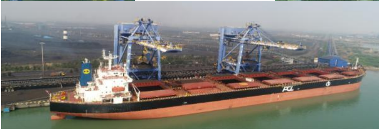
GSUs - 4 nos (Electric operated)
