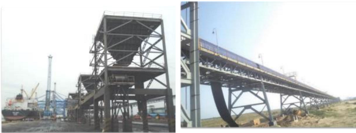
Hopper systems and Closed hood conveyors - mechanical handling systems
