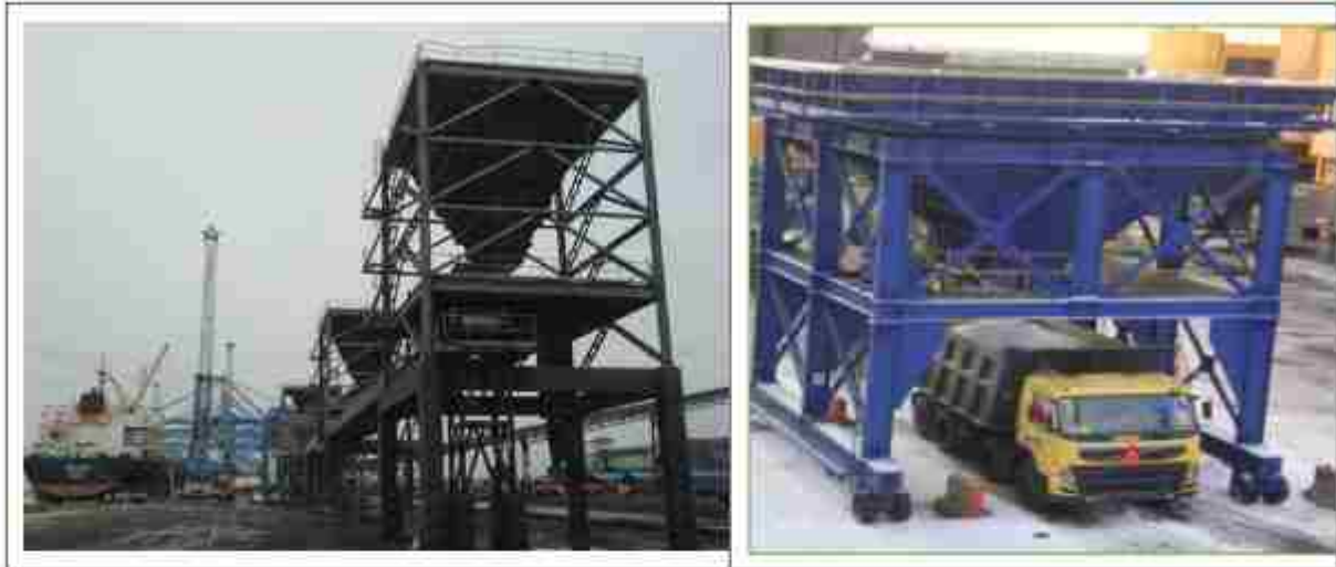
Figure 2:1 Mobile Hopper Reclaiming System
