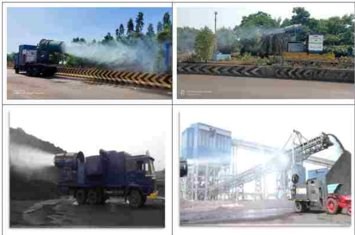
Figure 2:7 Atomizers in dust suppression system
