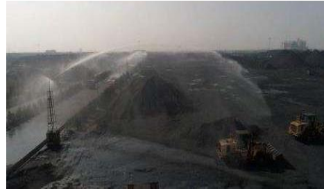
Dust suppression through Sprinkling system in AKPL
