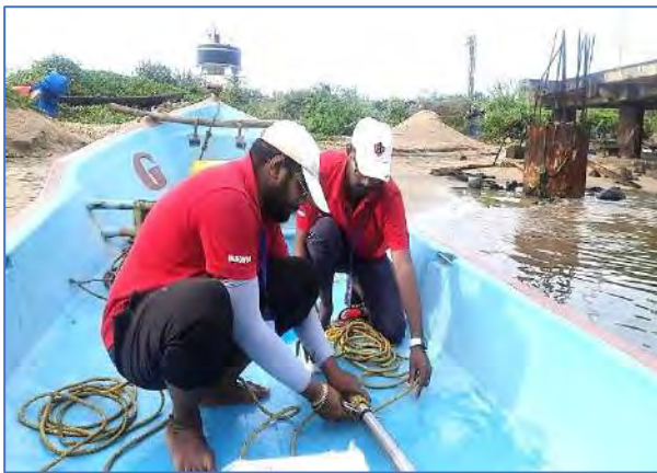
Installation of Transducer
