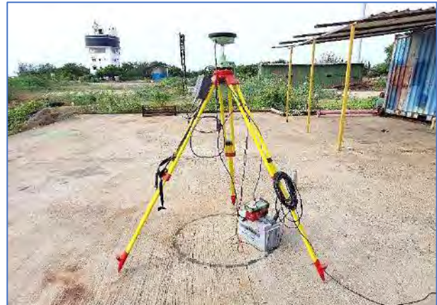
RTK Base station
