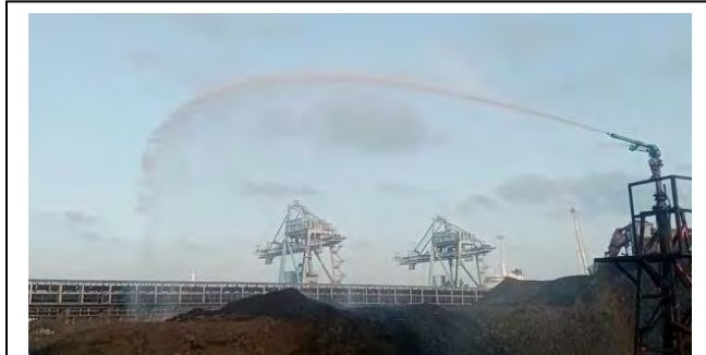
Sprinklers / Dry Fog Dust Suppression System
