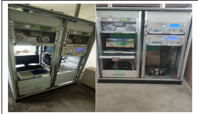
Automated Ambient Air Monitoring Stations & Display at Port Main gate
