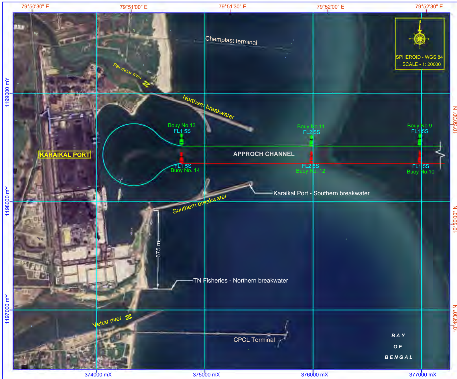
FIG. 2. ALIGNMENT OF TN FISHERIES BREAKWATER IN THE VICINITY OF THE KARAIKAL PORT BREAKWATER
