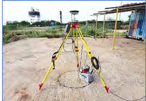
RTK Base station
