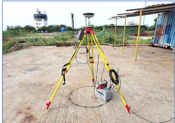
RTK Base station
