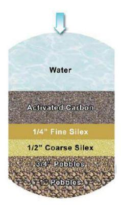
This filter uses the adsorption action of activated carbon.
