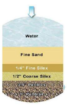
The upper layers of the sand perform the actual filtration function. The gravel layers merely provide physical support to the upper sand layers.
